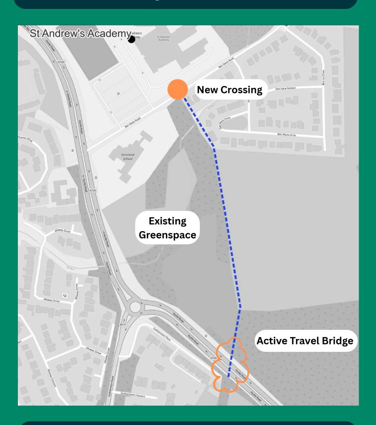
Option 1 would provide a shared use path following the old railway alignment, supporting coherence of the route and tying into Ben Nevis Road west of Ben Wyvis Drive.
