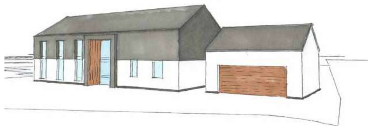
Option 1: zinc cladding render timber entrance feature
