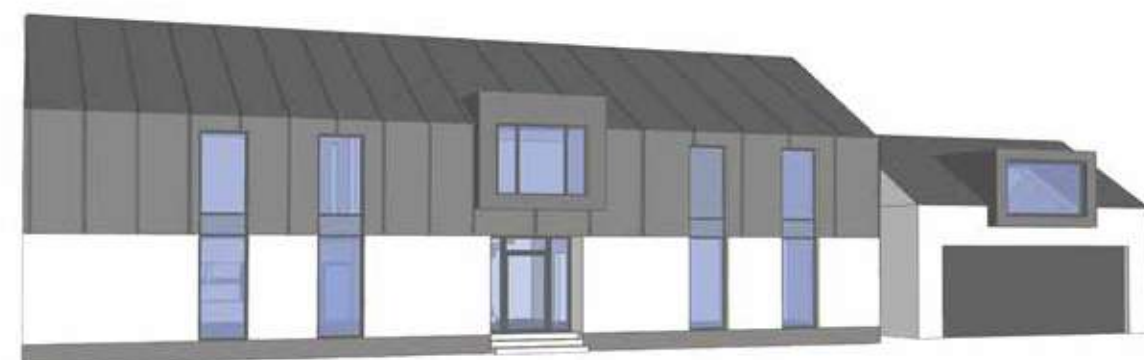
Option 4: long linear windows symmetrical single dormer on front elevation
