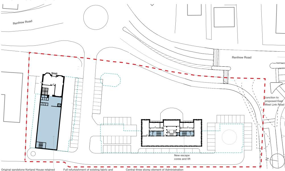
Original sandstone Kerland House retained and office extensions to east and south demolished and replaced with purpose built office accommodation Full refurbishment of existing fabric and services required (internal and external)
