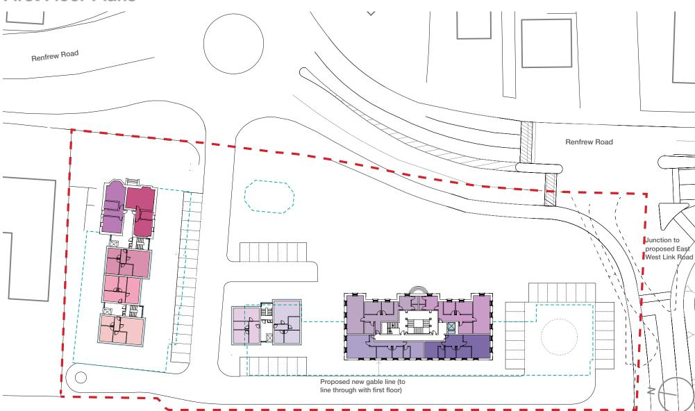
Original sandstone Kersland House retained and office extensions to east and south demolished and replaced with purpose built residential accommodation
