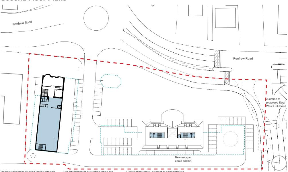
Original sandstone Kerland House retained and office extensions to east and south demolished and replaced with purpose built office accommodation
