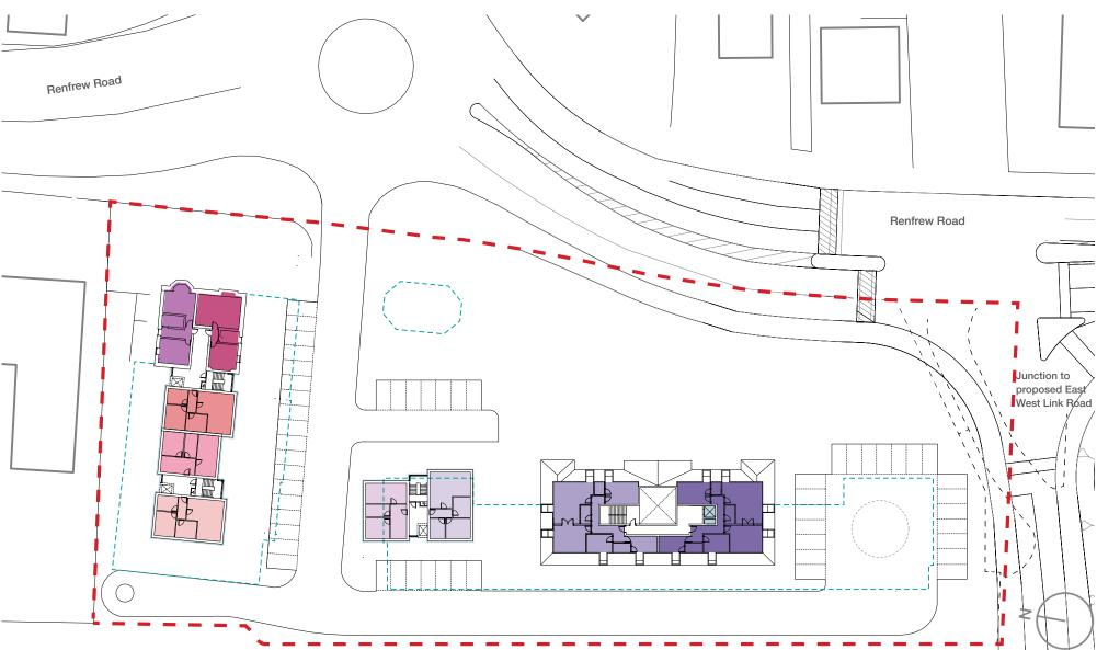
Original sandstone Kersland House retained and office extensions to east and south demolished and replaced with purpose built residential accommodation
