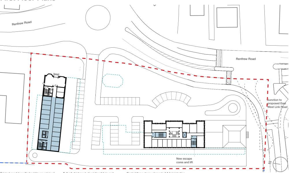
Original sandstone Kerland House retained and office extensions to east and south demolished and replaced with purpose built hotel accommodation Full refurbishment of existing fabric and services required (internal and external)
