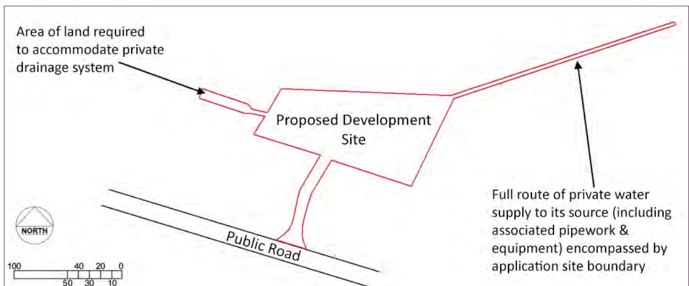
Fig 7. New private water supply and drainage arrangements
